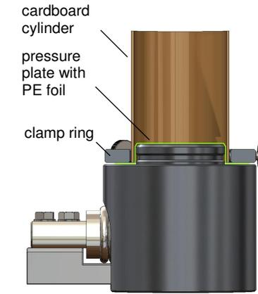
**Fig. 5:** Cross section of the new FPM 70, designed for the pressure measurement of high density foams.
