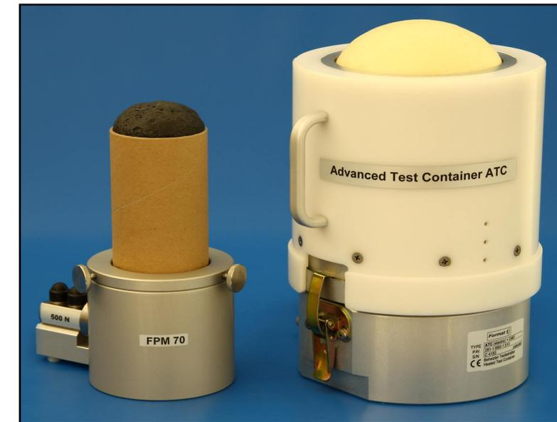
**Fig. 4:** The new Foam Pressure Measurement Device FPM 70 compared to the Advanced Test Container ATC. The test volume is reduced down to 15%.
