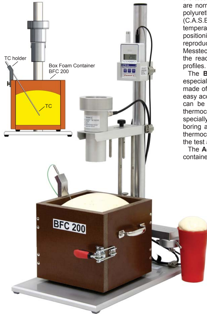
Fig. 1: The Box Foam Container BFC 200 is placed onto the base plate of the extended mechanical set. The metal sheathed thermocouple is inserted into the lower third part of the foam sample through a holder mounted at the upper edge of the BFC 200.
