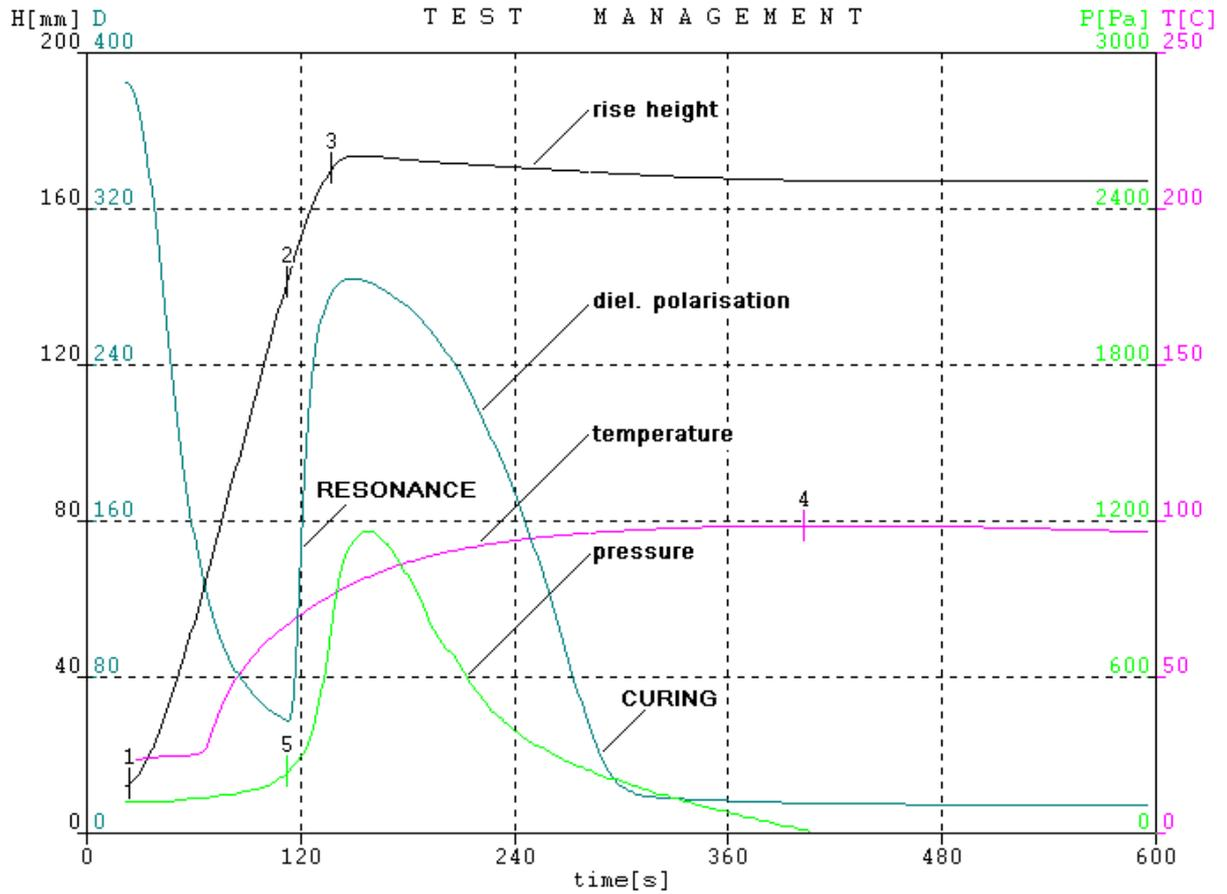
**Figure 2.** Dielectric polarization measured with CMD, and other physical data obtained for a molded foam. The polarization curve shows a significant resonance structure and the curing behavior.
