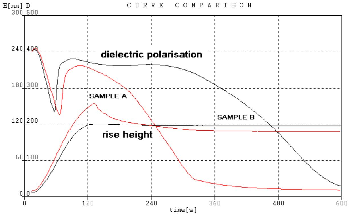
**Figure 2.** Comparison of the rise height and the dielectric polarization for two flexible foam samples with different isocyanate content. Sample B was made with 5/3 of the isocyanate amount of sample A.
