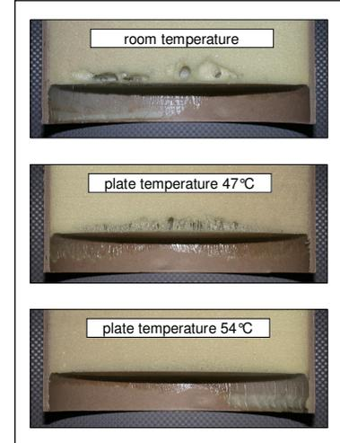
**Fig. 5:** Cross section of three samples of a flexible foam formulation, measured at three different bottom plate temperatures.
