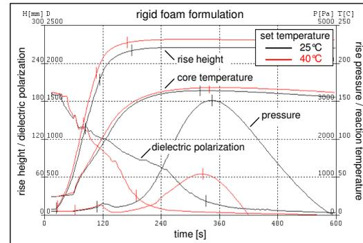
**Fig. 2:** Two sets of measurement curves of a rigid foam formulation, measured at different bottom temperatures of the test container. Depending on the temperature, the rise pressure and the dielectric polarization show most significant changes.
