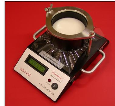
**Fig. 4:** The Pot Life and Curing Monitor Device SubCASE<sup>®</sup> and the high temperature test container filled with a white CASE formulation.
