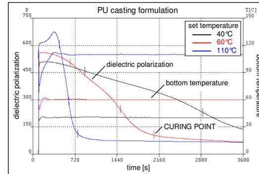
**Fig. 3:** Three SubCASE<sup>®</sup> measurements of a casting formulation measured at different bottom temperatures. The dielectric polarization shows strong temperature dependence: Curing goes faster with higher temperatures.
