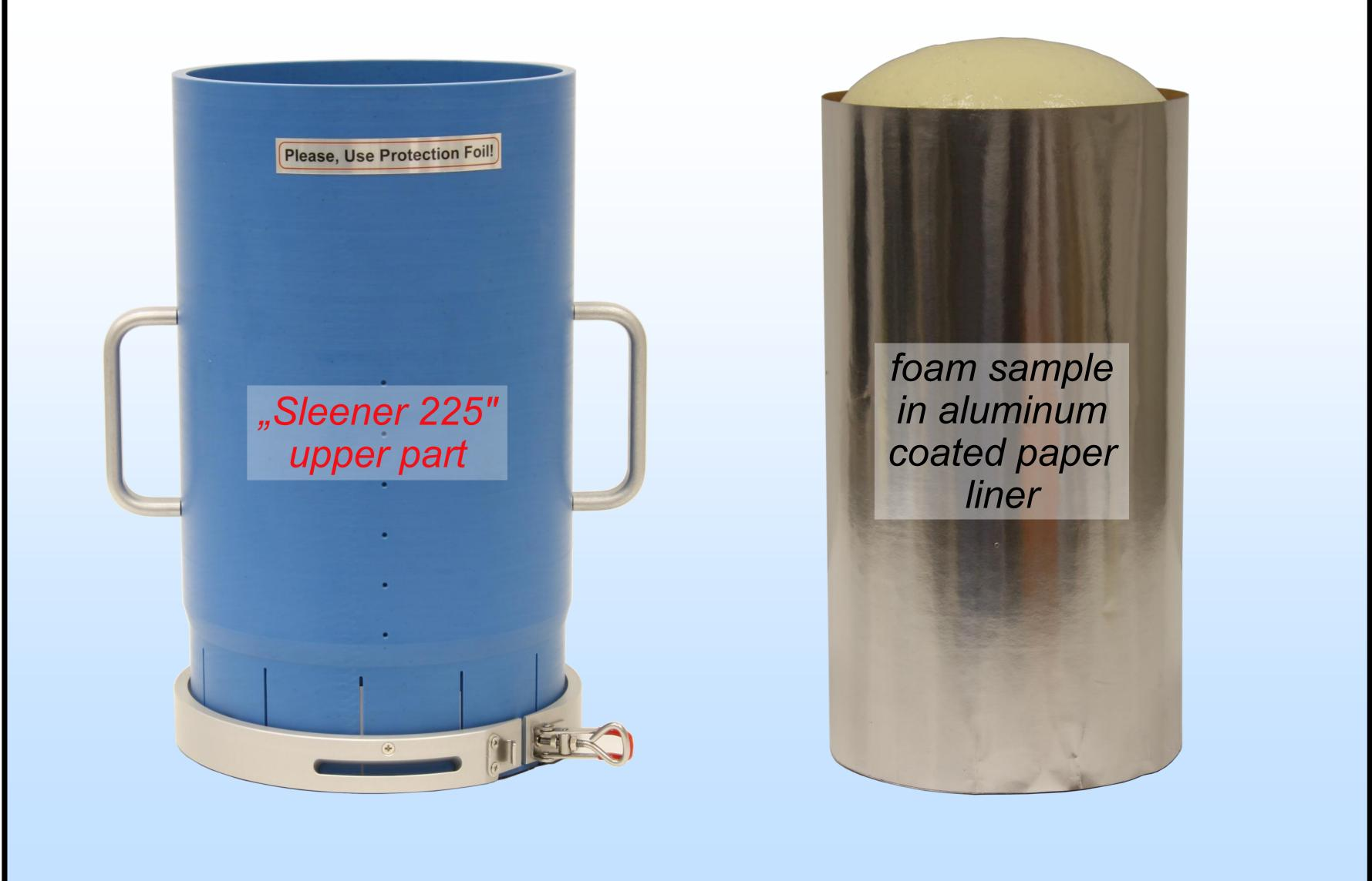
Fig. 4: The Sleener 150 has an inner diameter of 150 mm and a test volume of up to 5 liters. It replaces the Foam Pressure Measurement device FPM 150. No disposable cardboard cylinders are needed for each test.
