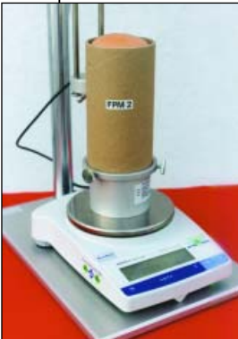
Fig 3 System for pressure monitoring
