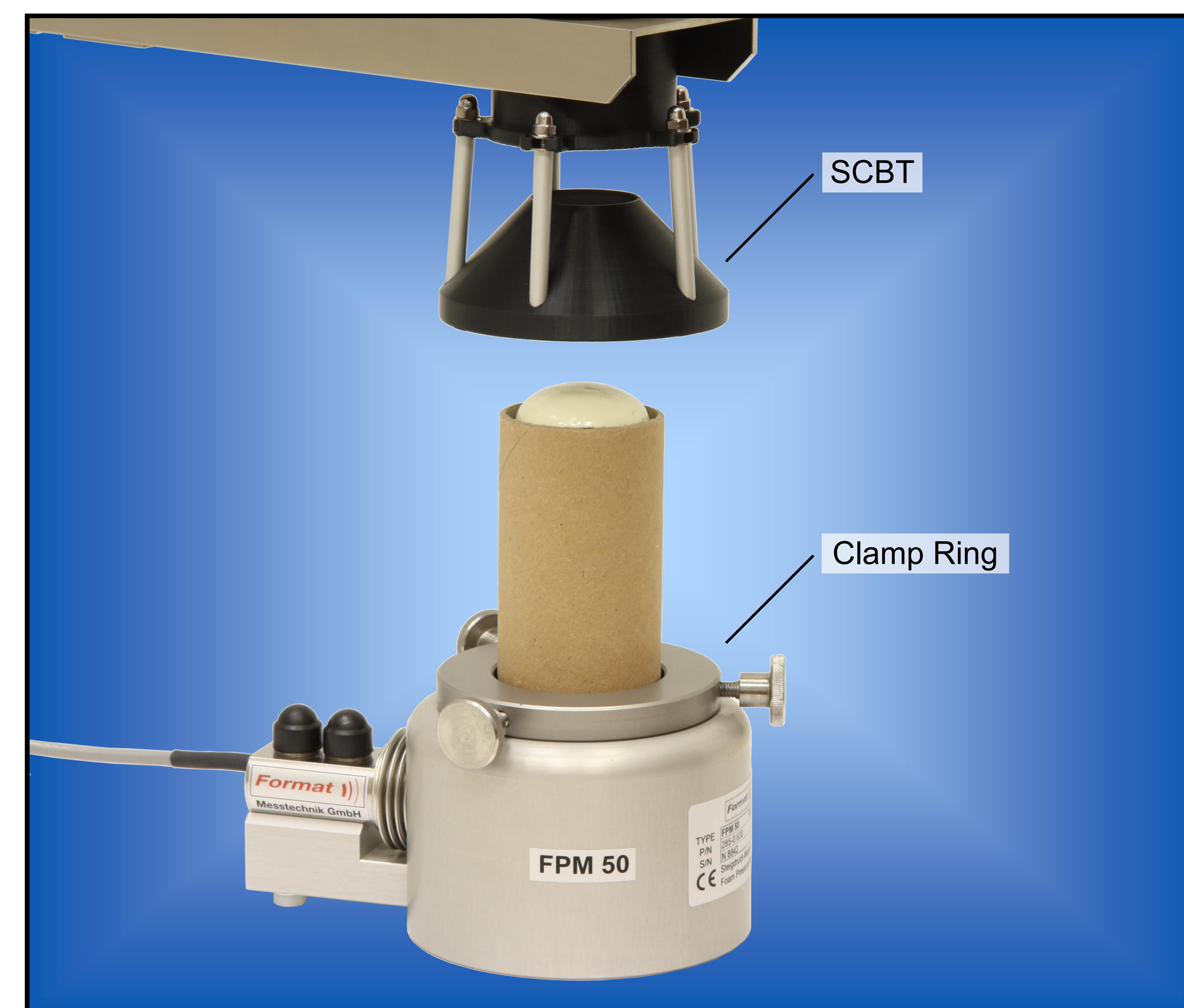
Fig. 4: The proofed ultrasonic fan sensor LR 4 with SCBT can be combined with the Foam Pressure Measurement device FPM 50 . This enables simultaneous rise height and pressure measurement.
