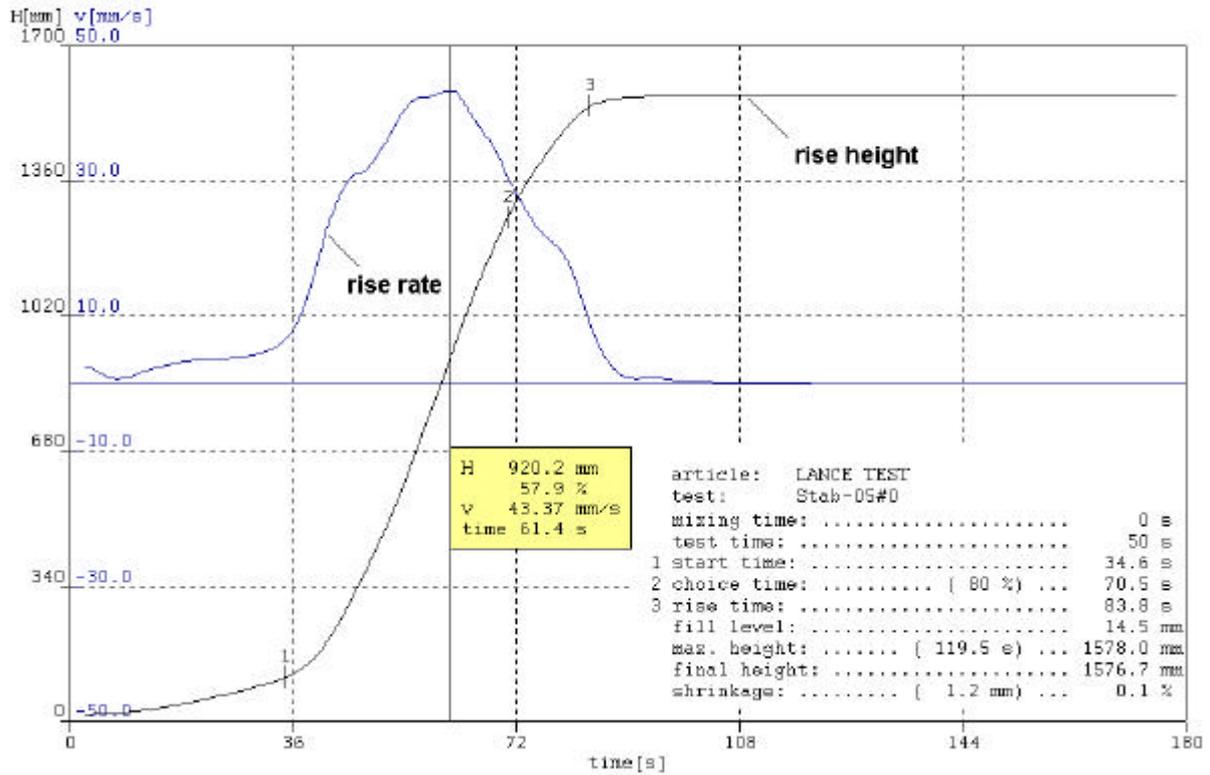
**Rise Height and Rise Rate of a Lance Test Evaluated by the Software FOAM**
