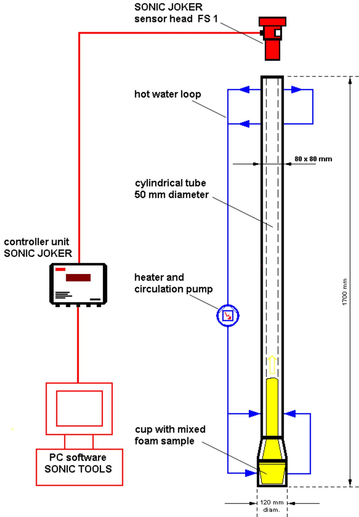
Drawing of the Lance Test Setup
