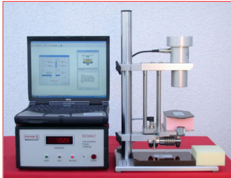
Fig. 1: Test device Resimat* for the measurement of the mechanical properties of viscoelastic foams. Left: Controller unit and software RESIMAT. Right: Ultrasonic sensor and hold/release mechanism.
